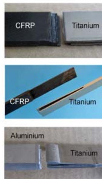
Figure 2. Different failure modes occurring in hybrid CFRP-Titanium-Aluminum transition structures after failure (Top: CFRP; Middle: hybrid laminate; Bottom: Aluminium (width 15 mm))[17]
