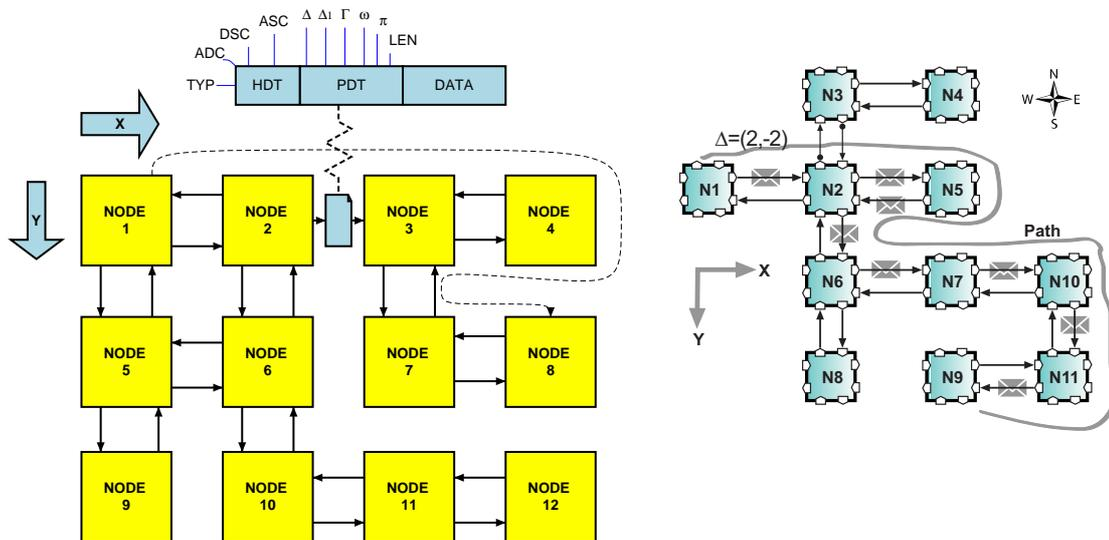
The main problem in message-based communication is routing and thus addressing of nodes. Absolute and unique addressing of nodes in a high-density sensor network is not suitable. An alternative routing strategy is delta-distance routing, used by SLIP. A delta-distance vector  $\Delta$  specifies the way from the source to a destination node counting the number of node hops for each dimension.
