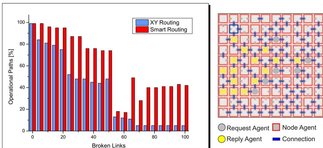
Results from stability analysis shown in Fig. 7 point out unstable behaviour under some particular network topologies. Though most situations are live
