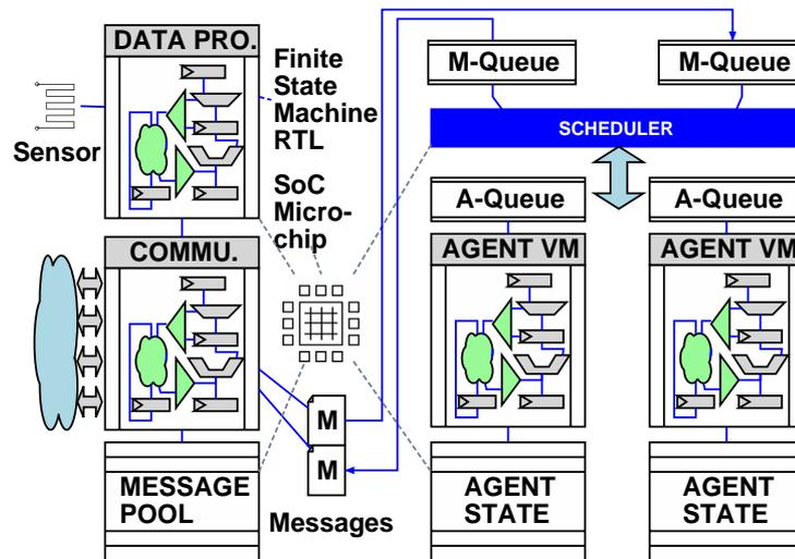
The functional agent behaviour is implemented with a (non-mobile) finite state machine (virtual machine) built in the sensor node, modelled with a high-level synthesis approach on an imperative multi-process programming language level [3].
